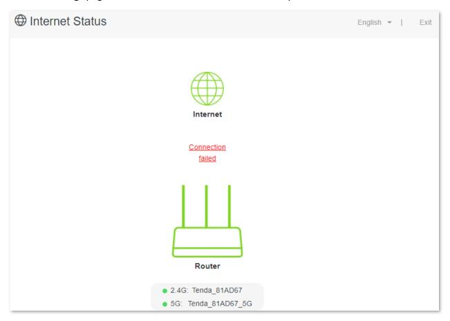
When "Please ensure that the cable between the Internet port of the router and the modem is properly connected" is shown on the page, ensure that the WAN port of the router and the LAN port of the modem or the Ethernet jack are connected properly. If the problem persists, contact the technical support for help.
